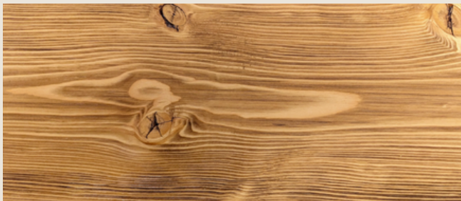
FIR TIMBER Exterior beams and fireplace mantel
